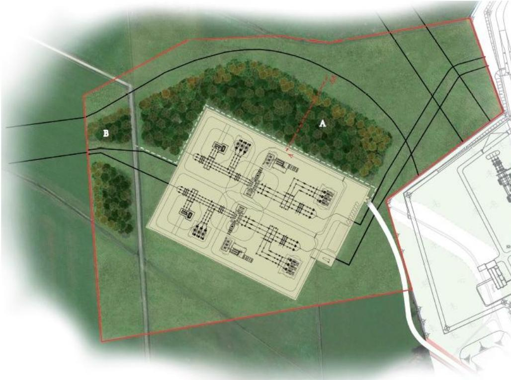
The substation has been designed to a scale appropriate for the capacity of the Wind Farm and the visible components will mainly be wires. The substation will have a maximum height of 11.5 m and an associated control building with a maximum height of 6 m.
