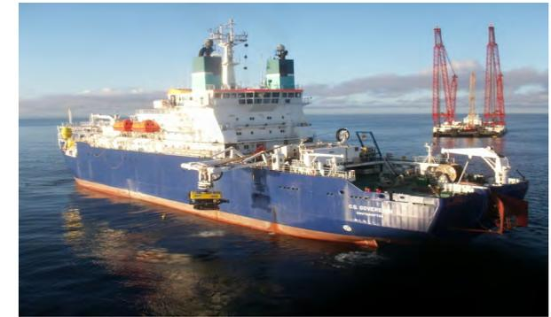
A typical cable laying vessel with cable trencher
